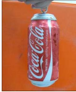
We all know what happens when you put liquids into the freezer- the coke can shows a dramatic picture of having the casing fully extended due to the water freezing!
